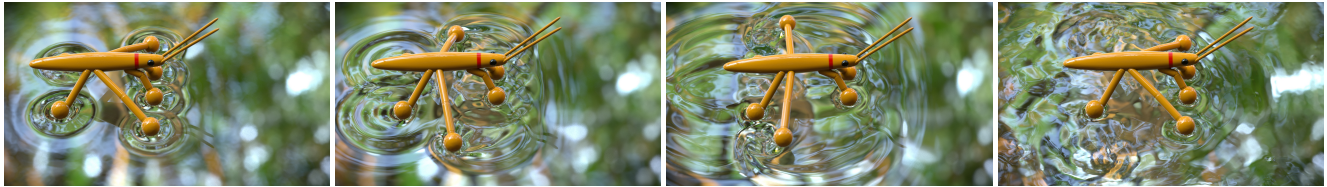
Fig. 14. Water Strider Robot. Our water strider robot is modeled using an articulated rigid body. We kinematically control its two middle legs to push down, push back and lift up sequentially. The reaction force cause by surface tension makes our insect robot move forward.
