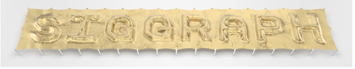
Fig. 8. SIGGRAPH banner. The eight letters are individually optimized as in the right of Figure 9b, and then their optimized material properties are assembled to form the banner.
